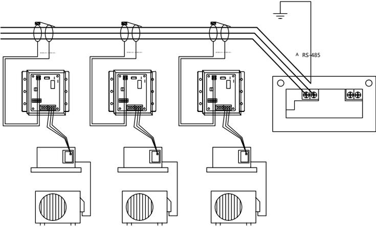
② the host equipment for the third party communication equipment, the detector provides the standard Modbusrtu protocol, BM1 dip switch: 1: ON; 2: OFF, The communication between the detector and the air conditioner is consistent with the other 3. When the detector is used as a third-party protocol converter, it should be specificAccess to the requirements of third-party host device connection; the basic functions are as follows:
