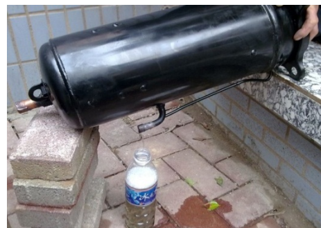
Figure 6-2.5: Draining oil from a compressor
